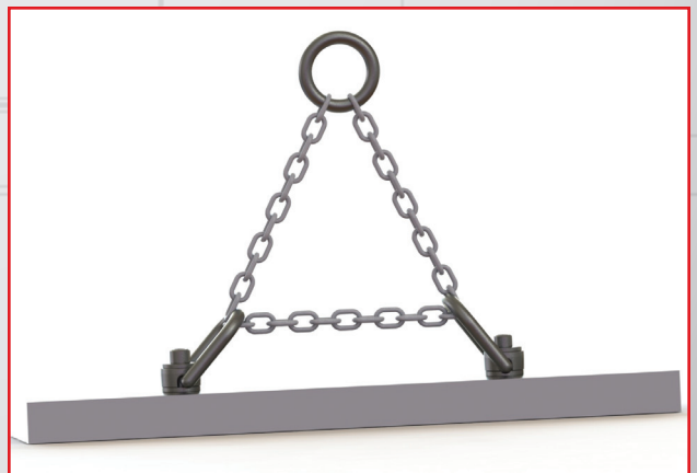
Unsafe Do Not Reeve
